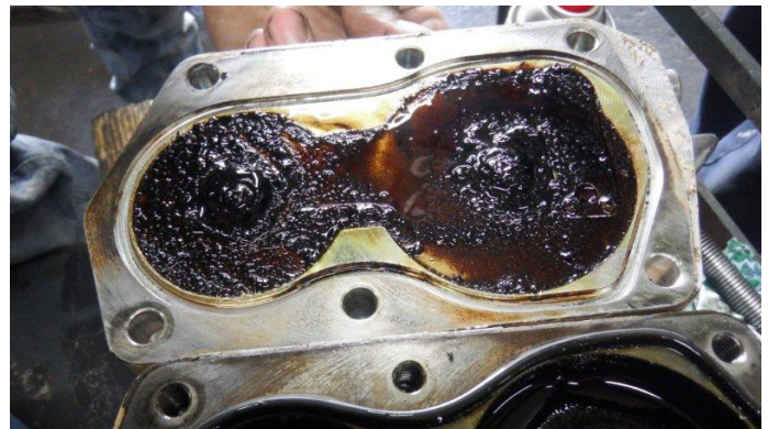
Above: Sludge build up resulting from incompatibility of mixed fluids.
